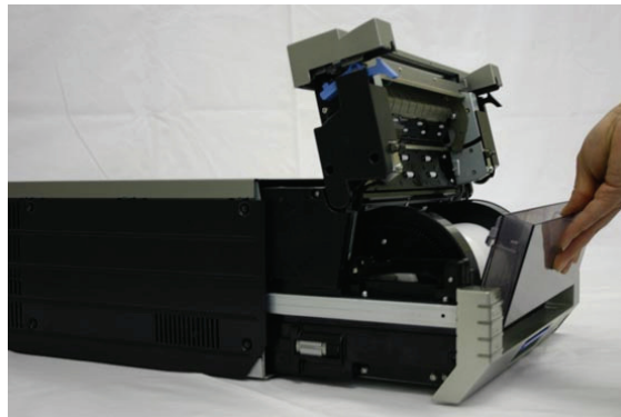
Figure 15. Removing the Scrap Bin
