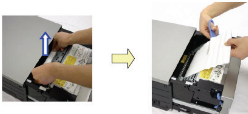
Figure 23. Pulling and Trimming the Paper
